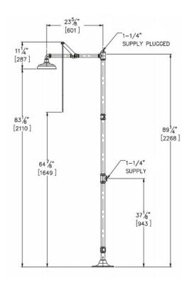
Model S2300 is our free standing safety shower complete with stainless steel shower head. Supplied with stainless steel pull handle, cast iron floor flange and 1" chrome plated stay open ball valve.
